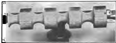
Fig. 52. Bead and Cove, Coves Completed.
